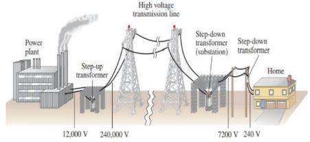
At generating station, normally voltage is stepped up to around thousands of volts. Power losses increase with the square of current. Therefore, keeping voltage high current becomes low and the loss is minimized.
